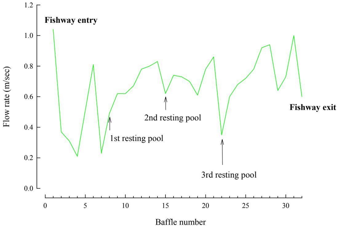
Figure 2 (A) The mean long-term monthly discharge (1964-2000) at the Goodga River Gauging Station and includes the spawning period of *Galaxias truttaceus*. (B) Flow rate within each concrete baffle (taken at the entrance to each baffle) of the Goodga River Fishway during May 2003.
